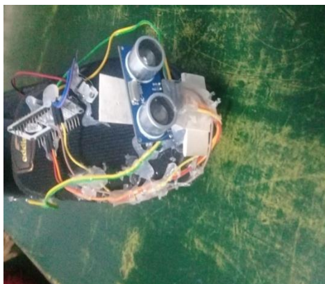
Fig 2 Proposed IoT-based Smart Shoes for Visually Challenged People
