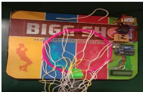
Fig 4 IR2 the second sensor ensures the count from below the hoop
