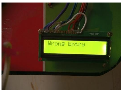
Fig 6 Activation of the buzzer signaling a foul as a result of an incorrect entry detected by the system
