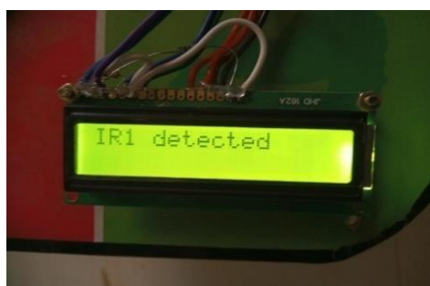
Fig 5 Count increase triggered by successful ball detection
